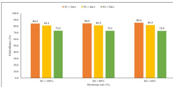
(c) Effect of discharge rate on field efficiency for different levels of forward speed for crop stage 1 (60 DAS)
