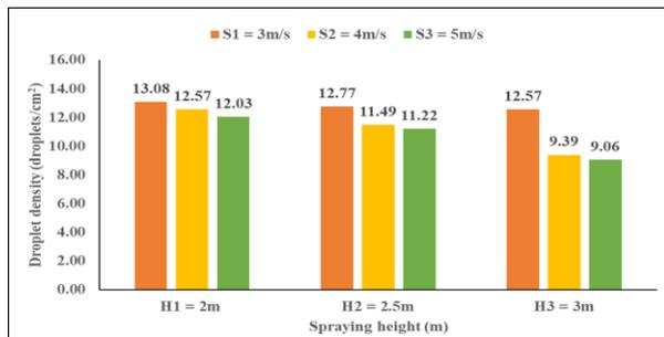
**(c) Effect of spraying height on droplet density for different levels of forward speed for crop stage 1 (60 DAS)**
