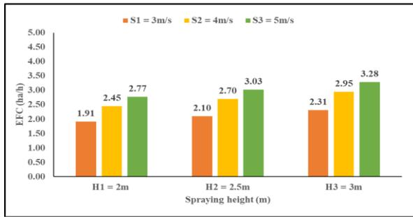
(a) Effect of spraying height on EFC for different levels of forward speed for crop stage 1 (60 DAS)
