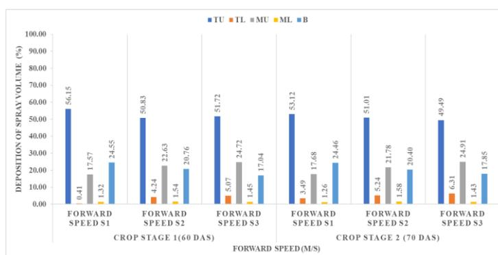
c. Percentage deposition throughout the plant at different level forward speed for crop stage 1 & 2
