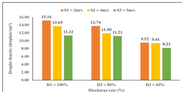
**(e) Effect of discharge rate on droplet density for different levels of forward speed for crop stage 1 (60 DAS)**
