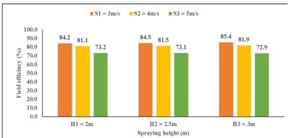
(a) Effect of spraying height on field efficiency for different levels of forward speed for crop stage 1 (60 DAS)
