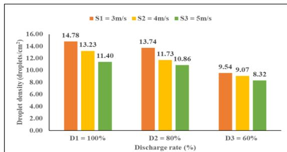
**(f) Effect of discharge rate on droplet density for different levels of forward speed for crop stage 2 (70 DAS)**
