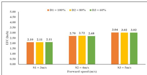
(c) Effect of forward speed on EFC for different levels of discharge rate for crop stage 1 (60 DAS)
