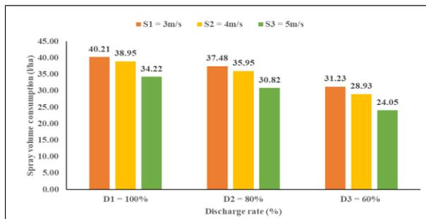
(e) Effect of discharge rate on spray volume consumed for different levels of forward speed for crop stage 1 (60 DAS)
