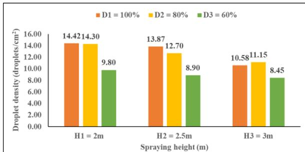
**(a) Effect of spraying height on droplet density for different levels of discharge rate for crop stage 1 (60 DAS)**
