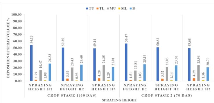
a. Percentage deposition of spray volume throughout the plant at different level of spraying height for crop stage 1 & 2
