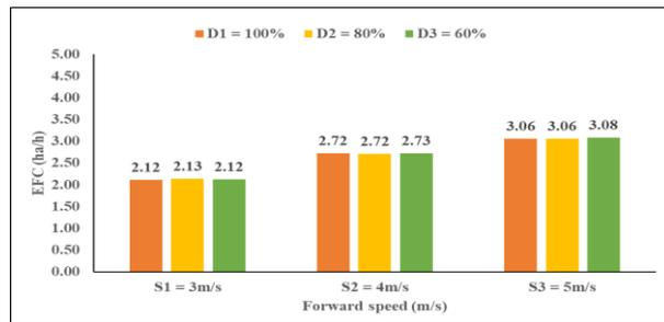
(d) Effect of forward speed on EFC for different levels of discharge rate for crop stage 2 (70 DAS)
