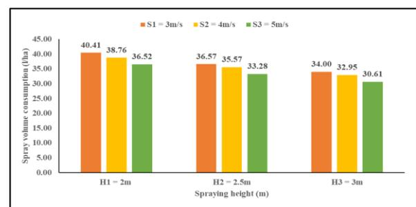
(d) Effect of spraying height on spray volume consumed for different levels of forward speed for crop stage 2 (70 DAS)
