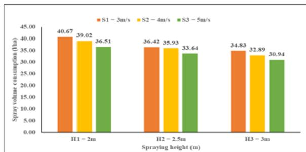
(c) Effect of spraying height on spray volume consumed for different levels of forward speed for crop stage 1 (60 DAS)
