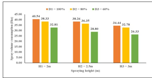
(b) Effect of spraying height on spray volume consumed for different levels of discharge rate for crop stage 2 (70 DAS)
