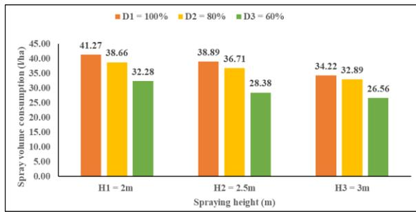
(a) Effect of spraying height on spray volume consumed for different levels of discharge rate for crop stage 1 (60 DAS)
