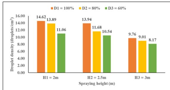
**(b) Effect of spraying height on droplet density for different levels of discharge rate for crop stage 2 (70 DAS)**
