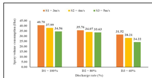
(f) Effect of discharge rate on spray volume consumed for different levels of forward speed for crop stage 2 (70 DAS)
