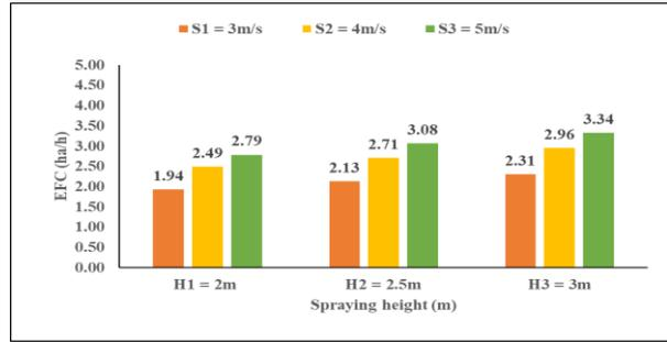
(b) Effect of spraying height on EFC for different levels of forward speed for crop stage 2 (70 DAS)
