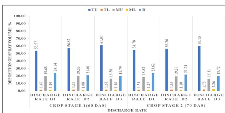
b. Percentage deposition throughout the plant at different level discharge rate for crop stage 1 & 2
