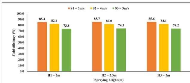
(b) Effect of spraying height on field efficiency for different levels of forward speed for crop stage 2 (70 DAS)
