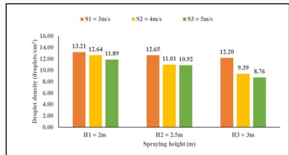
**(d) Effect of spraying height on droplet density for different levels of forward speed for crop stage 2 (70 DAS)**
