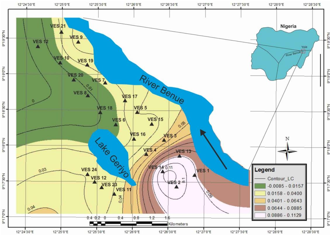
Fig. 4. Aquifer longitudinal conductance across the floodplain
