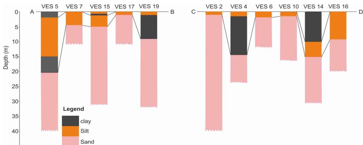
Fig. 3. The geoelectric section along AB and CD transect (in Fig. 1.) on the floodplain
